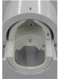
Volume Transmit, 32ch Array Coil Open for Subject Postiioning
