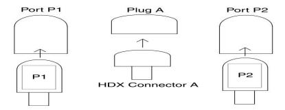
IMPORTANT: Always connect all three coil cables to the patient bed. Failure to connect all channels of array coil may result in coil damage and/or unsafe operation.
