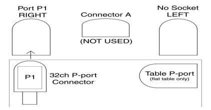
IMPORTANT: Always connect coil cables to the patient bed. Failure to connect all channels of array coil may result in coil damage and/or unsafe operation.
