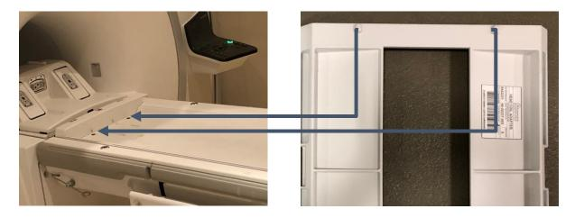
Place the Nova 3T 32 Channel Head coil on the table on top of the adaptor. The feet on sides of the coil fit into the recesses on the coil adapter.
