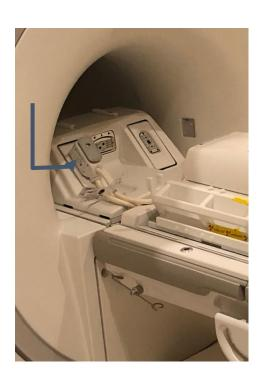
The Nova 3T 32 Channel Head coil has a built-in attenuation map which corrects for the gamma scattering caused by the coil. Consequently, it can be used during PET or simultaneous PET/MR acquisition.
